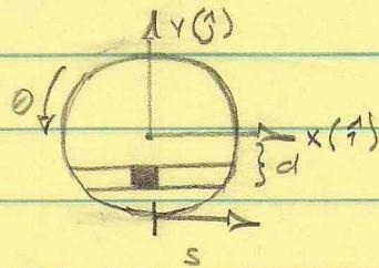
30 min q.i. write position of mass in terms of  $d, \theta, s$  using base vectors  $\hat{i}$  and  $\hat{j}$ . Differentiate twice.
